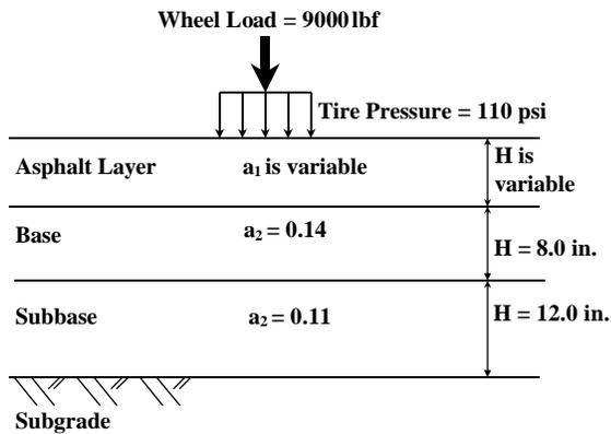
FIGURE 2 Pavement section used for comparative analysis.
